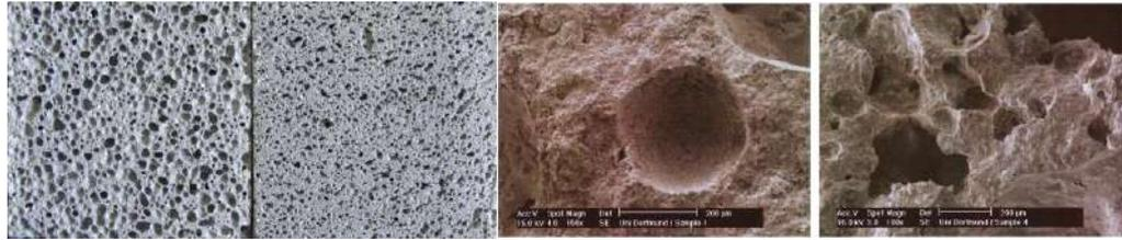
Figure 2.15. Foam concrete imaging (SEM and CT Scan) [25]
