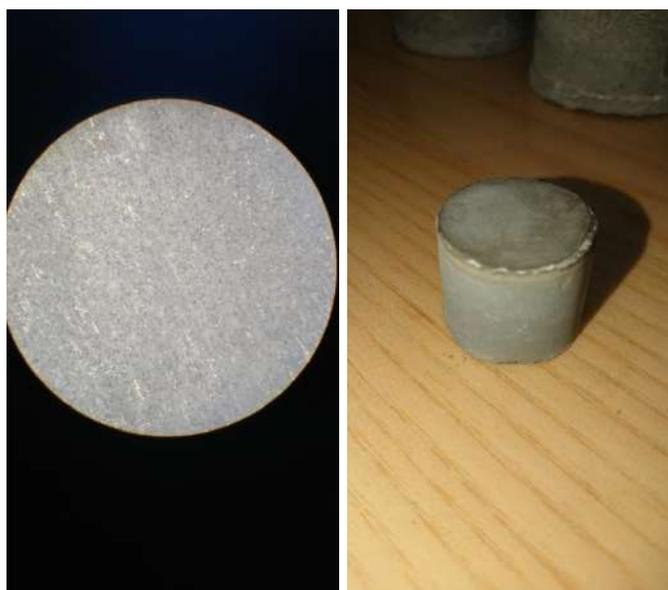
Figure 4.38. The image of net class G cement sample and its microscopic photography
