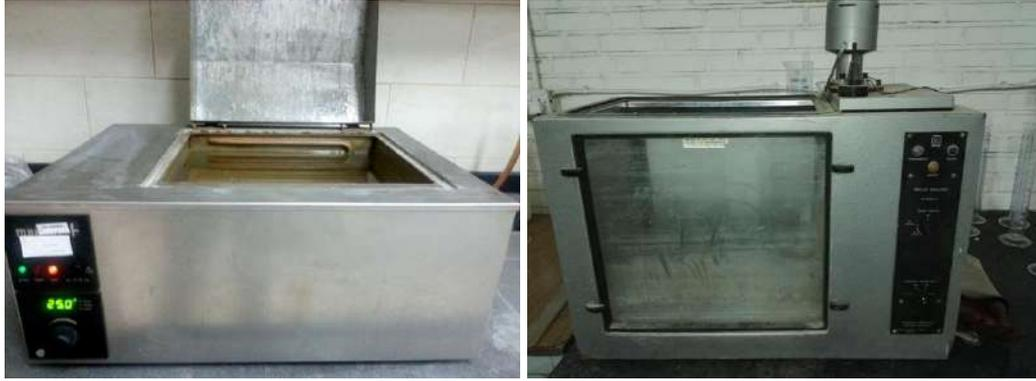
Figure 3.20. Two different water baths (PUT and NIDC's cement laboratories)
