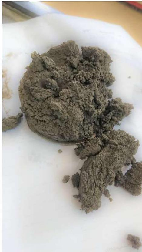
Figure 4.33. FBJ cement's cake after fluid loss test
