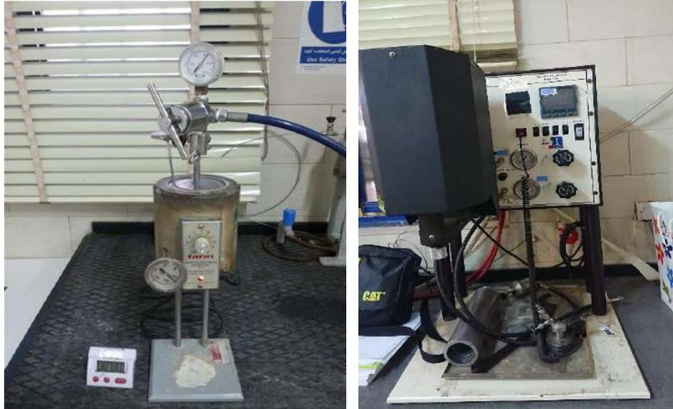
Figure 3.17. HPHT filter press cell (left) and a stirred fluid loss cell (right).
