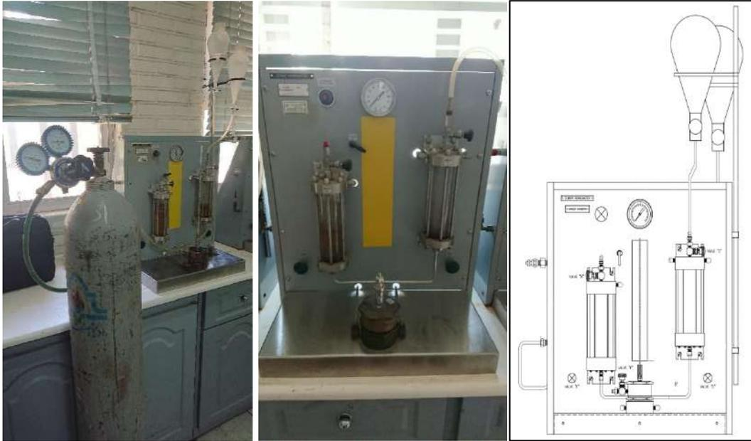
Figure 3.18. Photographic and structure of PUT's cement permeameter
