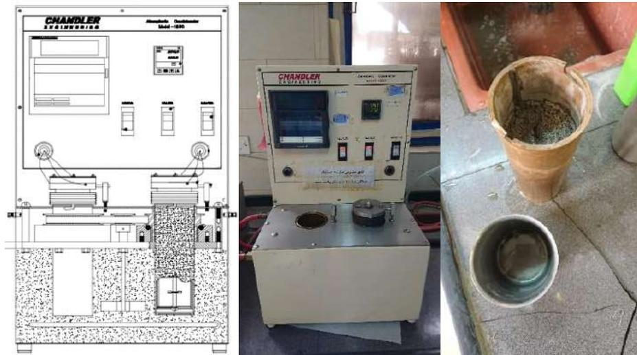
Figure 3.10. Photographic of atmospheric consistometer and its structure and cell
