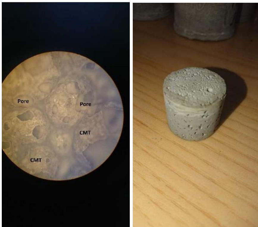
Figure 4.40. The image of OF+OR12 foamed cement sample and its microscopic photograph
