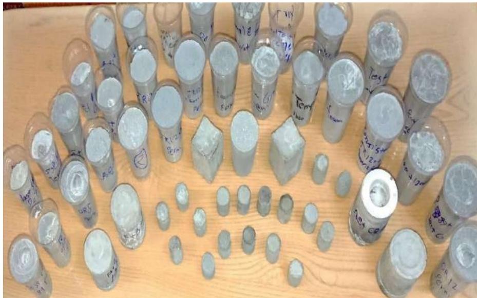
Figure 4.36. Some of the cement samples which prepared in surface or HPHT (210°F and 4000psi) conditions
