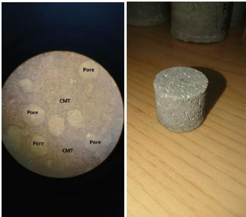
Figure 4.42. The image of FBJ foamed cement sample and its microscopic photography
