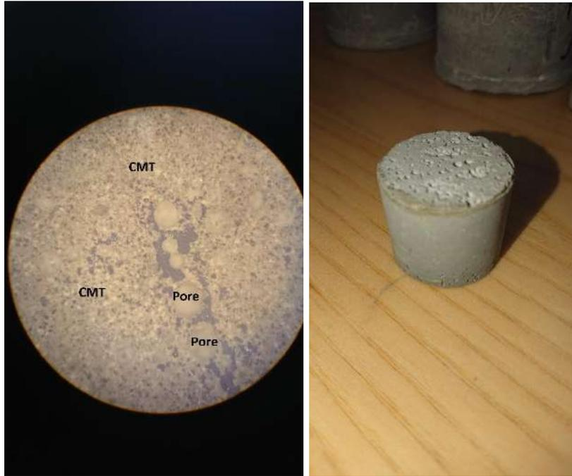
Figure 4.39. The image of OF+OR5 foamed cement sample and its microscopic photograph
