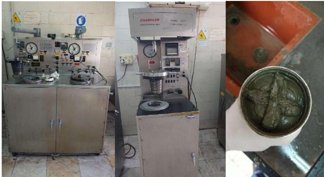
Figure 3.11. Two different HPHT consistometers and a thickened foam cement in NIDC's cement laboratory
