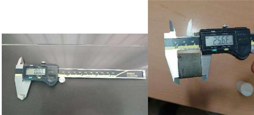
Figure 3.22. Digital Vernier Caliper
