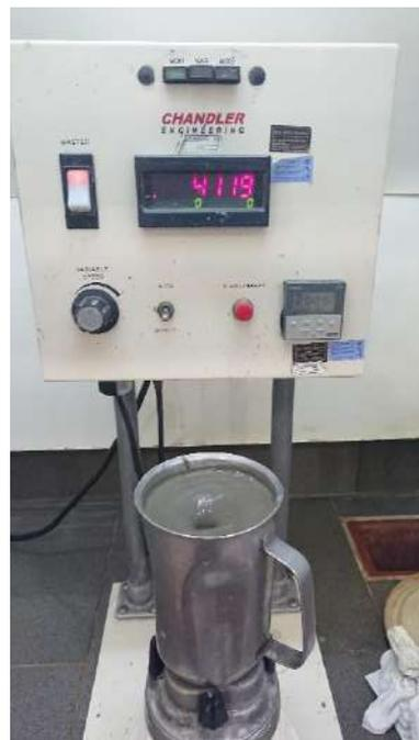
Figure 3.5. Photographic of NIDC's cement laboratory mixer
