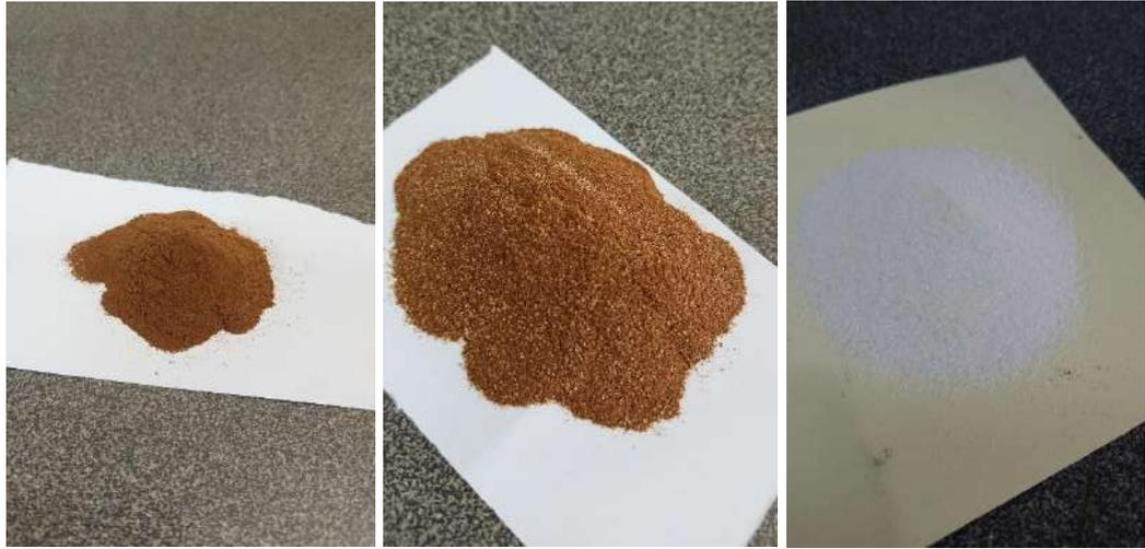
Figure 3.2. Different retarders that are used in this thesis, from left to right: OR5, OR12 and JR120
