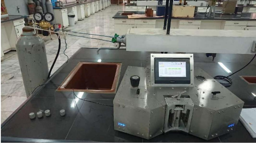
Figure 3.23. Image of PUT's petroleum laboratory helium porosimeter
