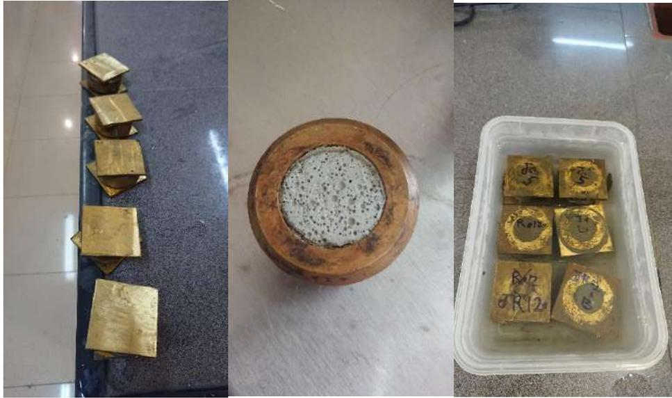
Figure 3.19. Cement permeameter molds and samples cooling procedure in the distilled water bath (rightest picture)
