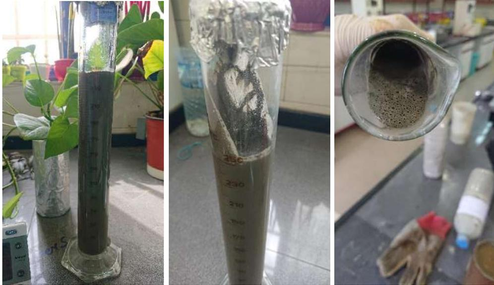
Figure 4.25. The photographic of free water and settling tests results on the FBJ slurry
