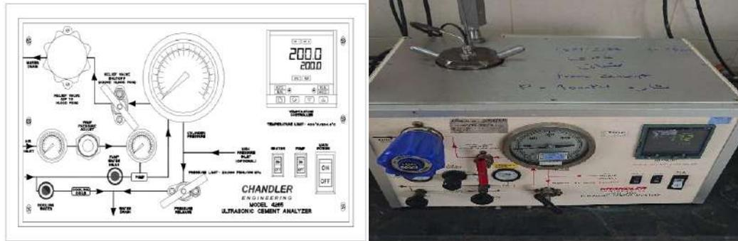
Figure 3.14. Photographic of UCA and its front panel
