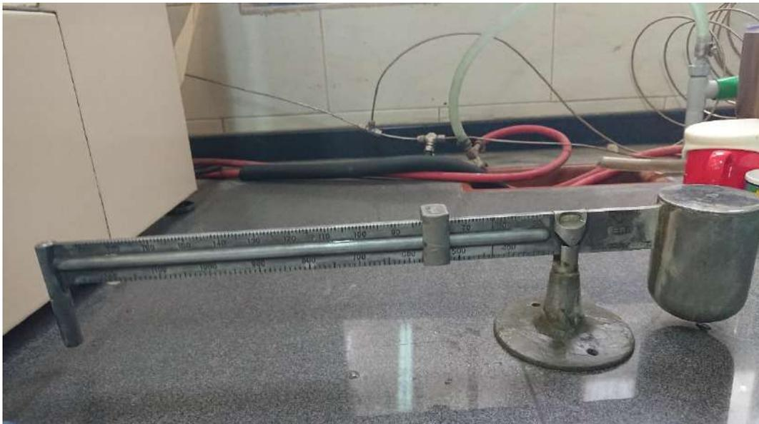
Figure 3.8. Image of NIDC's cement laboratory mud balance
